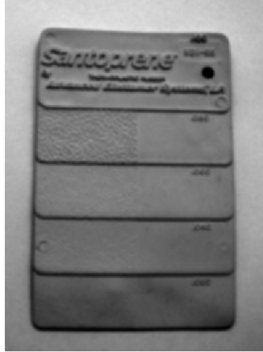
Figure 1.11 Thermoplastic elastomer with graded thickness
