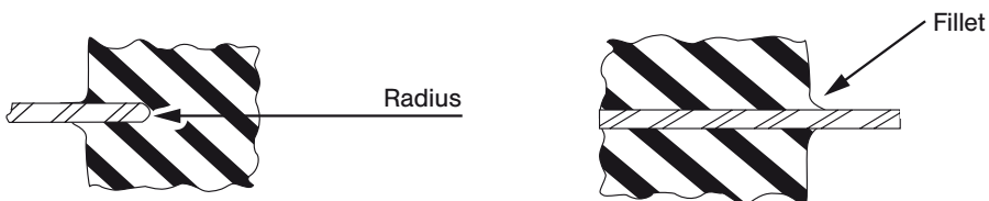
Figure 5.6 Radius or fillet in rubber and metal to reduce stress concentrations [21]
