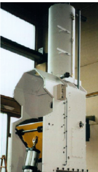
Figure 1.11 Pneumatic hopper assembly
