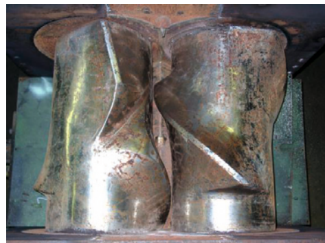
Figure 1.46 Intermeshing rotor by Wiedmann and Schmid [2]
