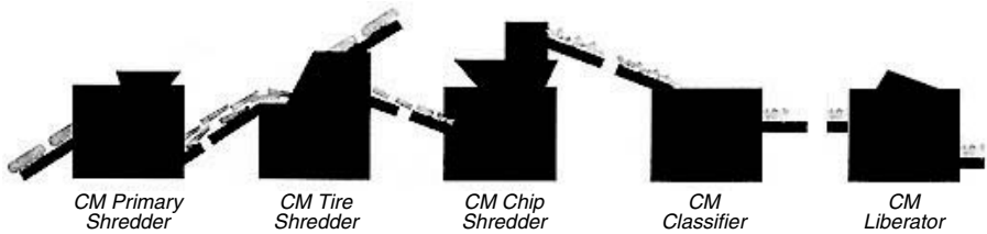
FIGURE 1.67 A turnkey wire and TDM system. 6,39
