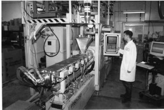
FIGURE 4.2 Research engineer Matthew A. Darling with production-scale PT-60 Berstorff pulverizer.
