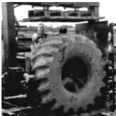
FIGURE 1.26 Tire balers with OTR tire and passenger tires. 19,20
