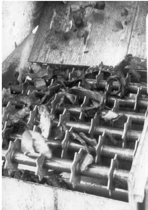
FIGURE 1.13 Tire chip production across a disk screen. 1
