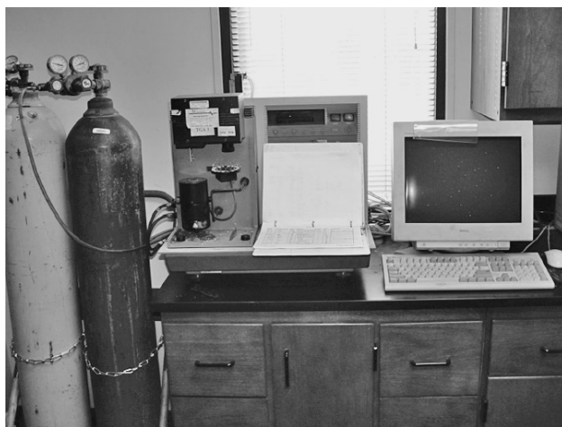
FIGURE 1.23 Thermogravimetric analyzer (TGA) laboratory set-up. 1
