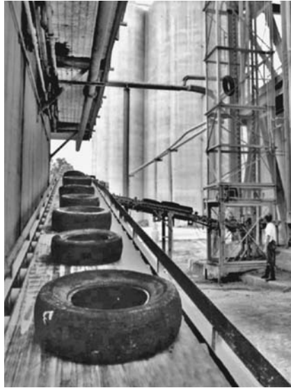
FIGURE 1.8 Whole tire metering unit for a cement kiln application.
