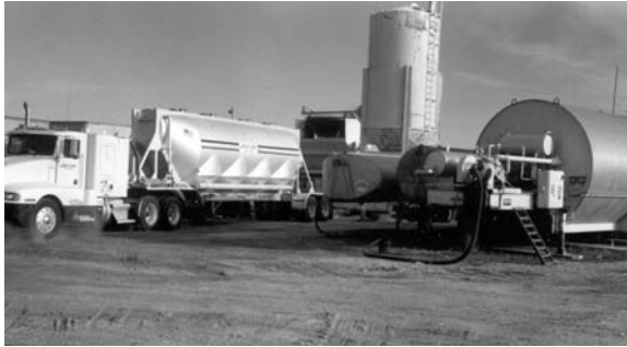
FIGURE 1.83 An actual asphalt facility using a bulk delivered minus 80-mesh CRM. 1
