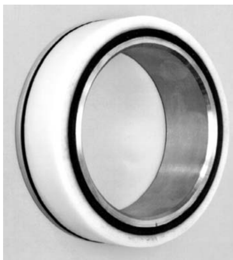
Figure 5.5 Thrust reducer used to decouple the submarine propeller shaft. The natural rubber is sandwiched between the steel ring and an outer layer of polyethylene
