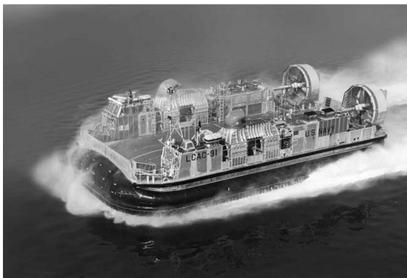
Figure 5.17 Landing Craft Air Cushion propelled by two four-bladed 3.7 m diameter, variable-pitch propellers. The polychloroprene/Nylon tube can be seen at the water interface
