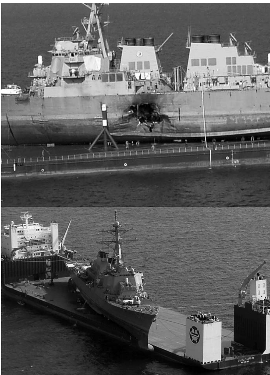
Figure 5.2 The guided missile destroyer USS Cole being returned to the United States after a terrorist attack in Yemen in October 2000. Despite the 150 m 2 gash in the port side of the hull (upper photograph), as well as the jostling when the ship was mounted on a salvage transport vessel, the bow dome (seen in lower photograph hanging off the edge of the transport) was still functional. After repairs that included replacement of 550 tonnes of exterior steel plating, the Cole returned to sea duty 18 months later
