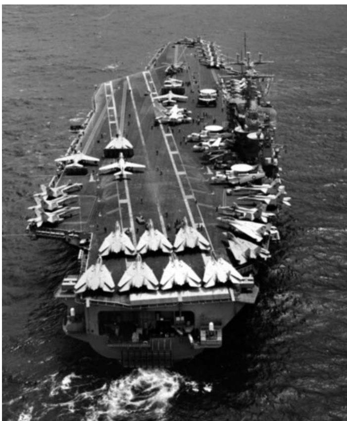
Figure 5.12 Nimitz-class aircraft carrier, the world's largest warship. Manoeuvring required to position planes for launch is responsible for much of the tread wear
