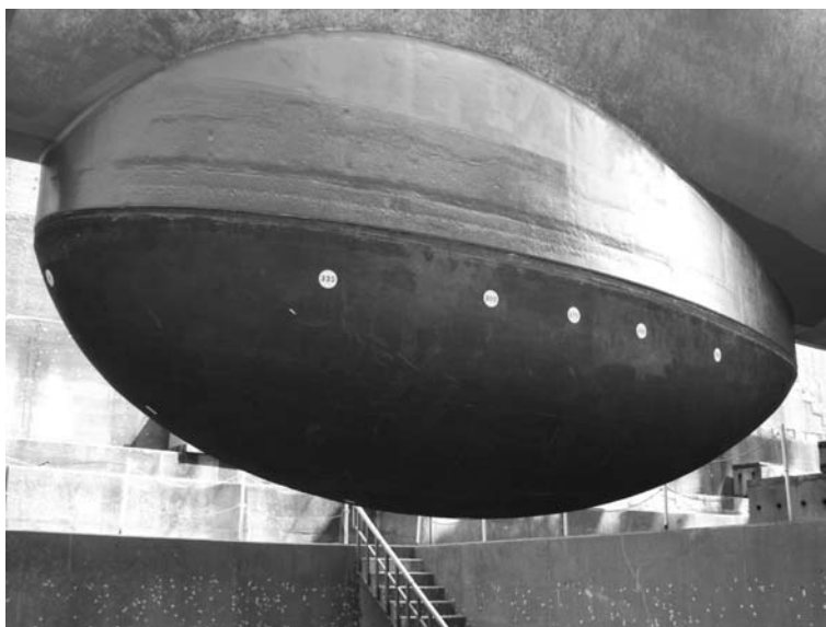
Figure 5.4 Composite keel dome composed of two resin-impregnated fiberglass outer layers and a soft rubber core. The geometry of the structure is tuned to be acoustically transparent over a limited frequency range
