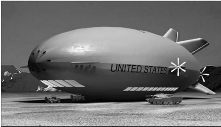
Figure 5.14 Artist's conception of the giant blimp WALRUS intended for rapid strategic airlifts
