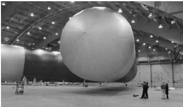
Figure 5.15 Prototype space blimp, 53 m in length, being float tested Photograph courtesy of J.R. Aerospace; www.jpaaerospace.com
