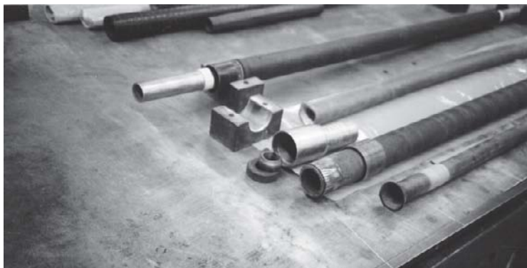
Figure 8.18 Pressure hoses (and assembly items)
