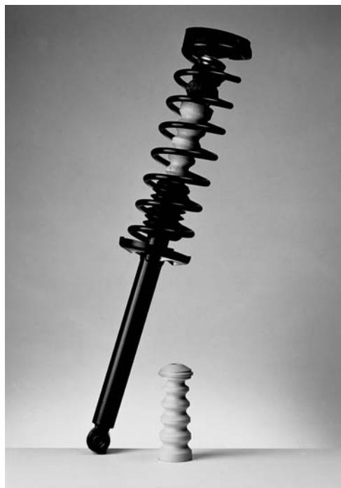
Figure 15.56. Elastic element for shock absorber (Courtesy Bayer MaterialScience LLC).
