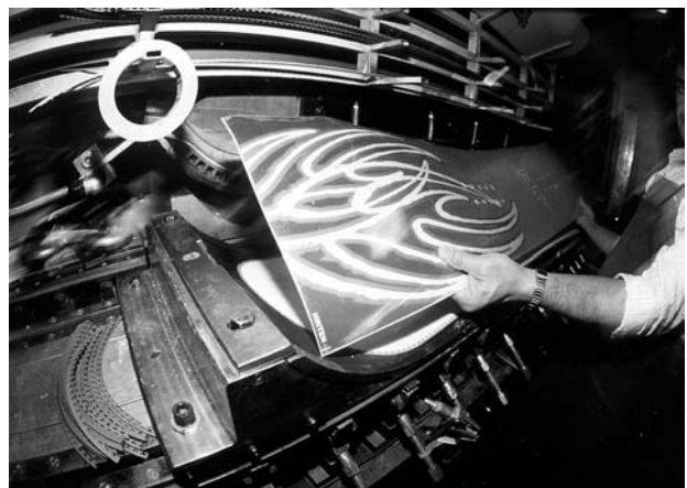
Figure 15.85. Molding of a snowboard (Courtesy Degussa AG).
