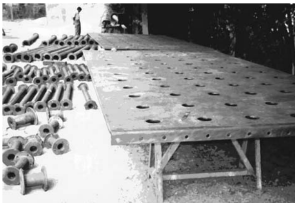
Figure 3.4b Rigid mild steel rubber lined cell cover
