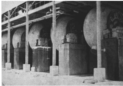
Figure 4.2 Rubber lined spherical digesters in an ore industry
