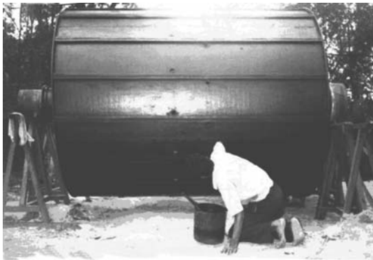
Figure 7.3 Rubber lined filter drum fixed with division strips
