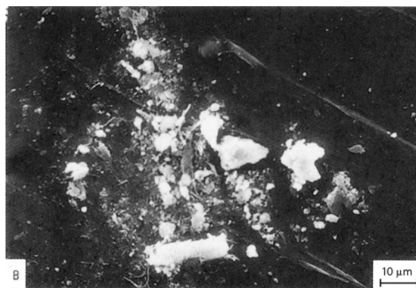
Figure 12.15 Scanning electron micrograph of compounds 4(A), showing many undispersed particles, and (B) undistributed particles.
