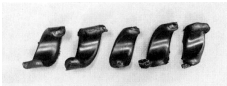
Figure 12.5 Patches of Passenger Tyre Tread (PTT) rubber compound removed from screw.
