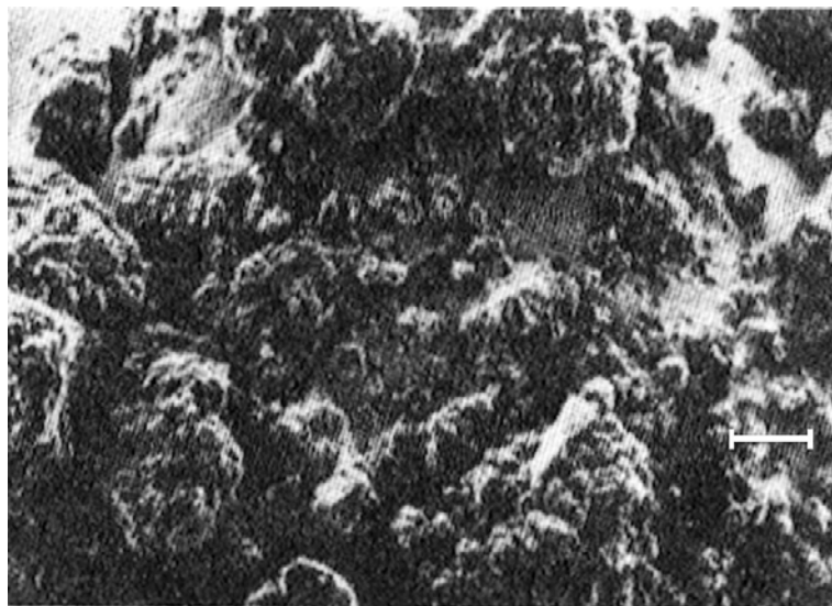
Figure 9.12 Scanning electron micrograph of N330 carbon black after mixing or crushing for one minute. Scale bar 100 \mu\text{m} .
